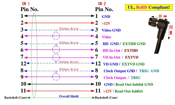
For Some CCD Model, Pin (8,9,10,11) are just no connections, and Cam Cable assy with this connection is fully applicable!
